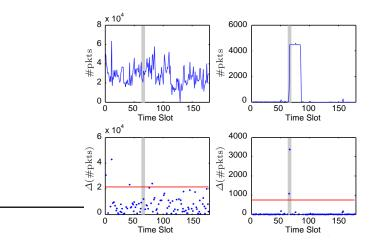
Fig. 2. Low-intensity anomalies might be hidden inside highly aggregated traffic, but are visible at finer-grained aggregations. The DDoS attack is evident at the victim's network.
