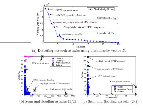
Fig. 4. Detection and analysis of network attacks in MAWI.
